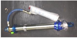
New 2.5 king coil over shocks, 14" stroke shock, remote reservoir with compression adjustment clickers and internal triple bypass, part # RS2514- COHRS coils are available as well. \$630 each tim@cpiresources.net
